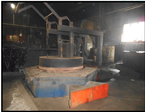
Fig 3.6 Tempering process Furnace in heat treatment plant
